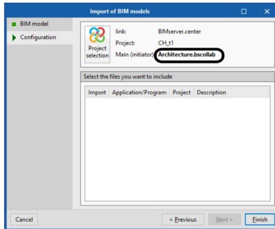
Figure 10: Importing Cype Architecture Model from BIMserver.center. Screenshot of OpenBIM Analytical Model.
