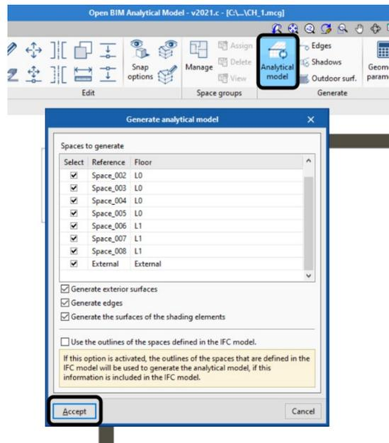
Figure 11: Generating the Analytical Model. Screenshot of OpenBIM Analytical Model.
